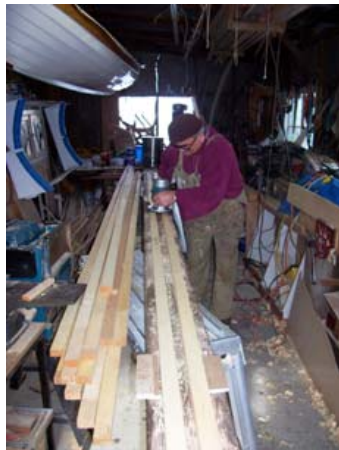
Huon rib preparation underway!
