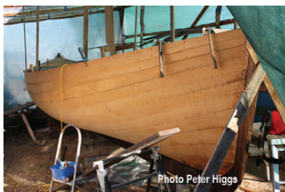
Photo Peter Higgs All planking complete
