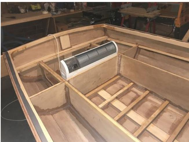
Over the last month, added the final floor timbers, and I've made and installed the knees, laminating them out of strips of left-over hoop pine. A pattern was made and fine-tuned, and this was then used to make a jig that I could clamp and bend the glued strips against.
