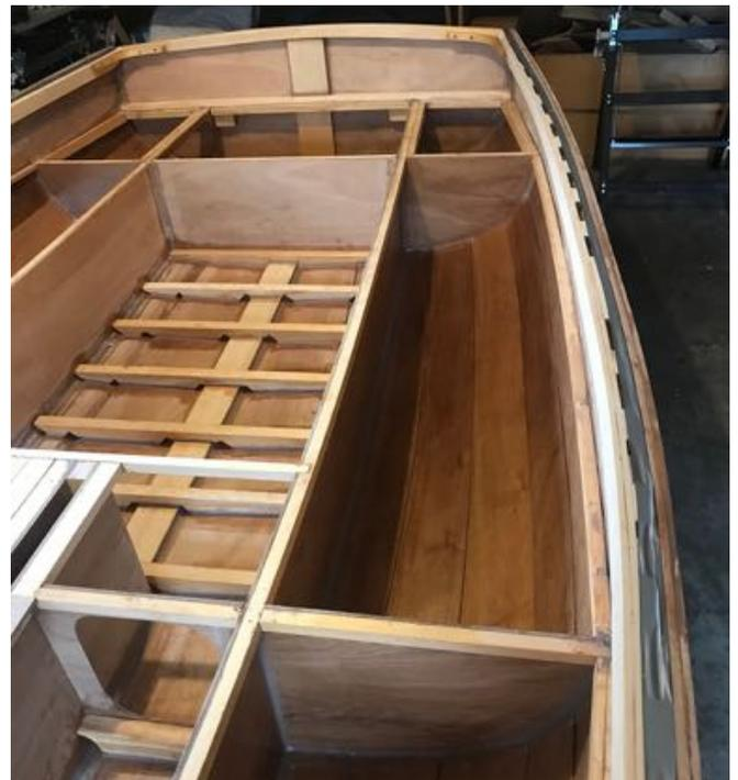
The boat is now upside down again, and the base of the centreboard case has been finished, with the sides cut to level with the inside of the case, using a router and a rasp, and then sanded, epoxied, and taped.
