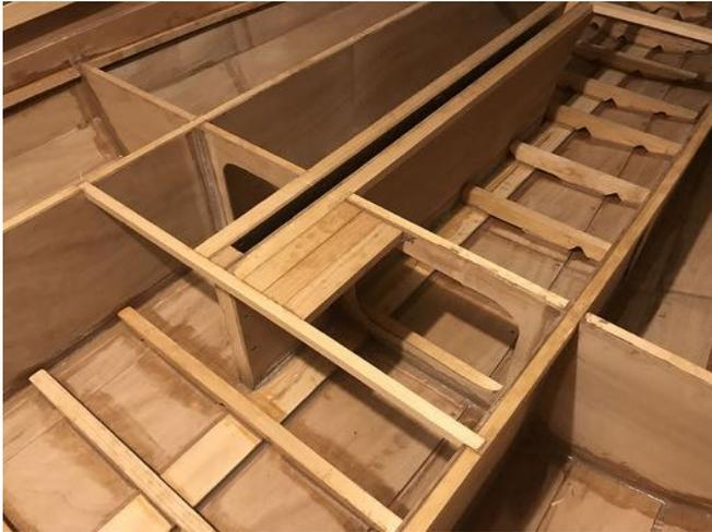
Then it was on to making and fitting the stringers that will support the seats against the hull. Resting a level across the longitudinal bulkheads, I scribed a line along each side of the hull, marking where the stringers had to be fitted. Wedging everything in place, I completed marking the position of each stringer, and once they had been removed I epoxy coated these areas along the hull. The stringers were then glued up and fitted into the hull.
