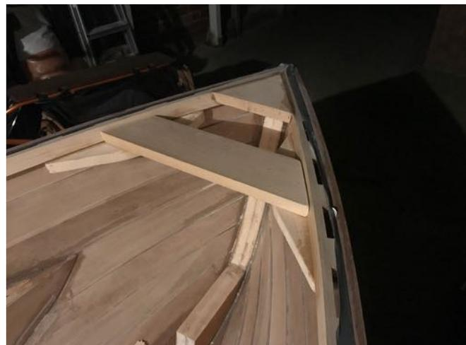
I've glued up the pieces that the Mizzen mast will slot through, once I cut the appropriately sized hole, and fitted them in between the stringers that will support the thwart at the aft end of the centreboard case.
