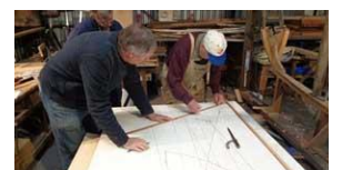
Use the batten strike the oblique line on the plank table
