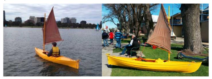
**One person sea kayak**, 5.2m long by 0.6m wide. Fast and stable with fore and aft hatches. Stitch and glue construction with hoop pine for the bottom and sides and gaboon ply for the deck and a lifting rudder with foot controls.
