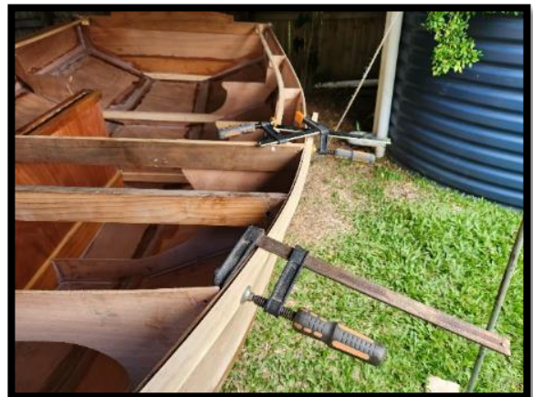
Dick's interior framed
