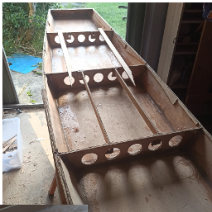
Above: Deck stingers layed out. Also note the rough cut inwales out of offcut materials
